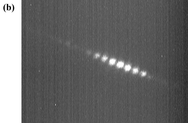
Figure 3. (a) Setup for free space diffraction imaging in a low voltage TEM, and (b) the resulting diffraction pattern.
